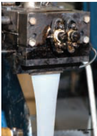
Intimate mixing of polymers by Readco Extruder equipped with vertical sheet die.
