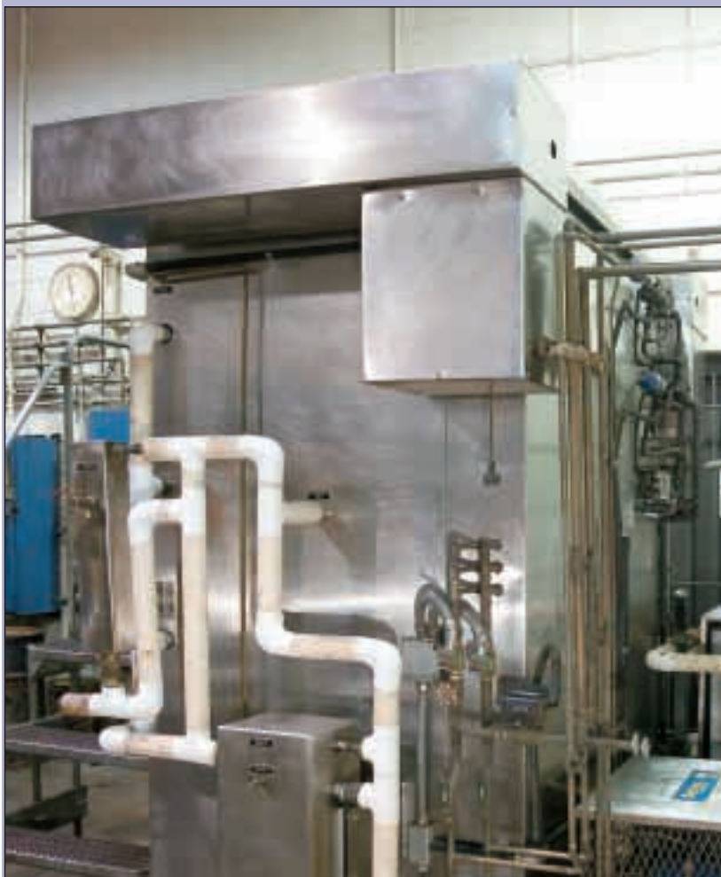
Detrex vapor degreaser is seven-foot-tall and totally cleans all parts sent to Winston for processing.
