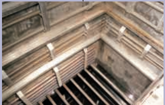
Empty vapor degreaser work basket. Contaminated parts are preheated in this basket by a system charged with Paratherm NF heat transfer oil before vapor degreasing.
