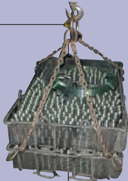
Basket of cleaned parts immediately after being removed from the vapor degreaser.
